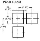
Note: Recommended panel thickness is 1 to 3.2 mm.
